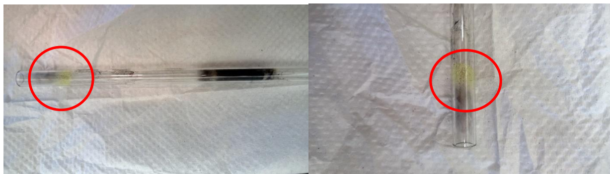
Figure 7.9: Yellow S deposited (marked by red circle) at the outlet when nano-iron oxide (HD-2 and HD-3) was used as a catalyst.
