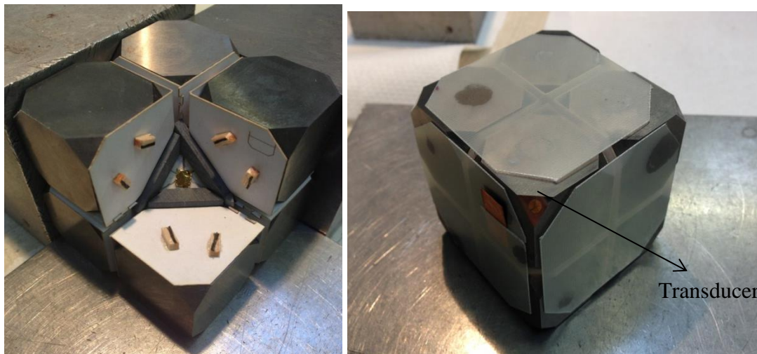
Fig. 2.4. The final assembled MgO octahedron and eight WC cubes.
