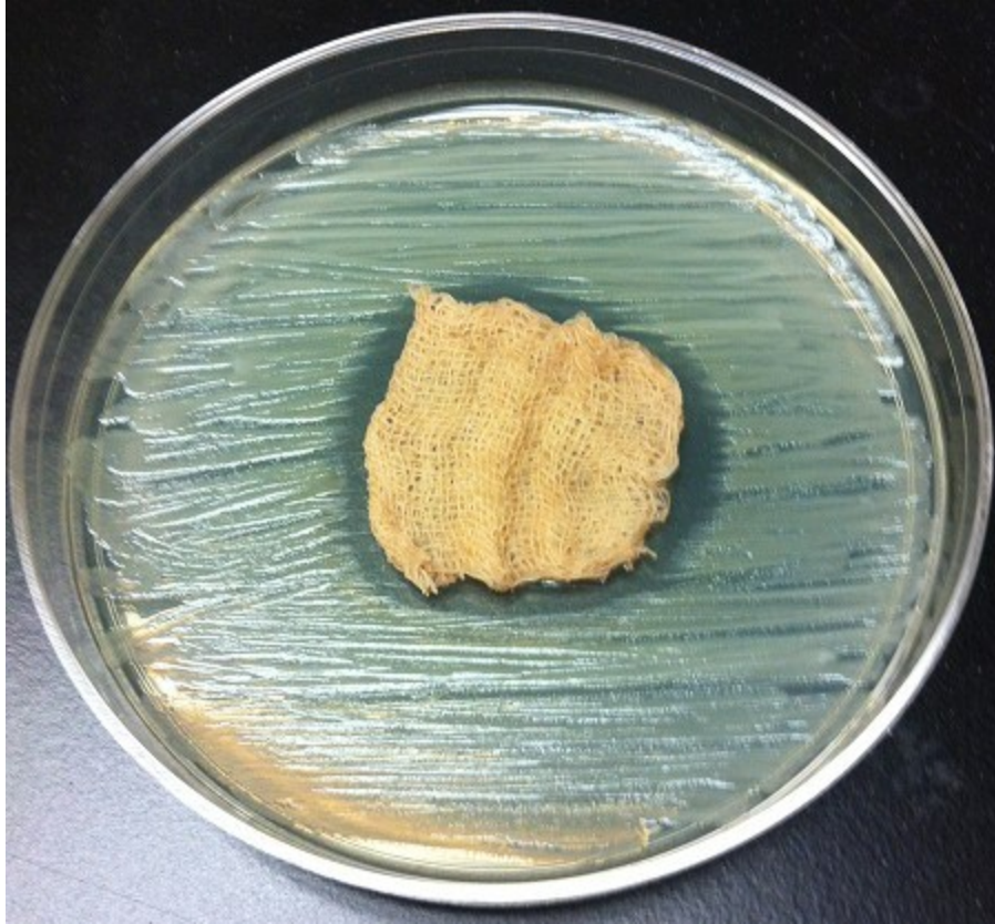
Fig.26 The zone of inhibition around bandage pre-treated with proanthocyanidin-loaded chitosan-TPP nanoparticles on Day 2
