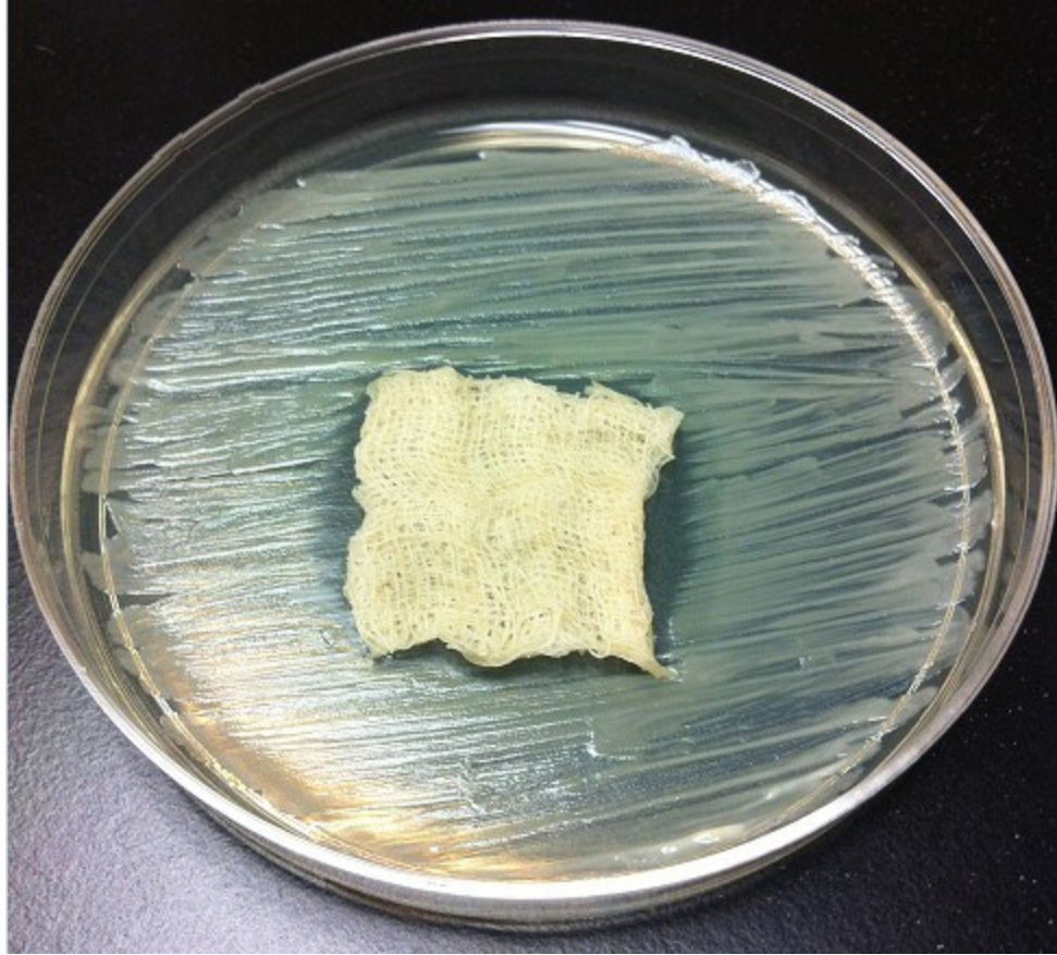
Fig.24 The zone of inhibition around bandage pre-treated with chitosan-TPP nanoparticle on Day 2
