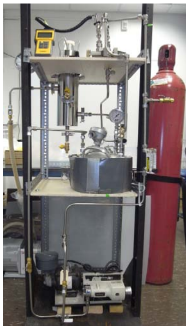
Figure 2-15 (a) Schematic representation of the pervaporation apparatus, (b) actual set-up of the unit. Also shown is the gas tank on right.
