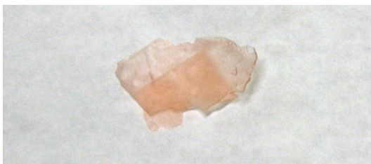
Figure 8-1 – Clear coating PU-1 (MIL-53039) after exposure to solvent system D for 2h with subsequent drying, showing a purple tint indicative of impure solid phenol.
