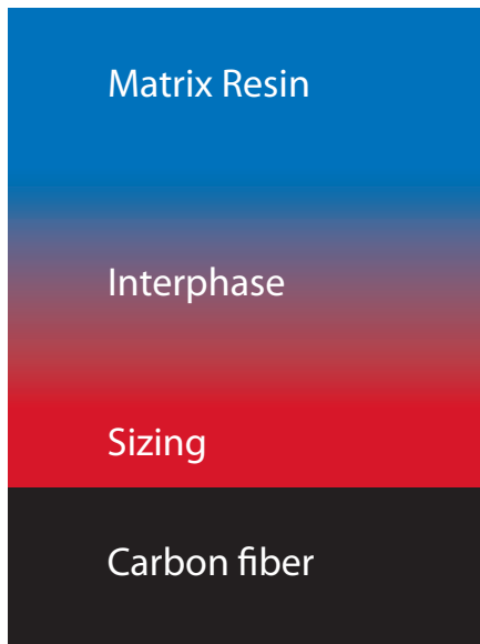
Figure 2-5 – Schematic representation of the carbon fiber - sizing - matrix interphase region
