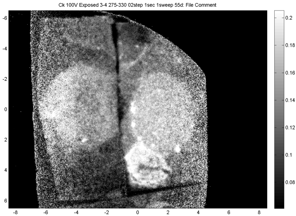
Figure 9-12 – Pseudocolored hyperspectral image of PhOH/H 2 O-exposed, fully-formulated MIL-PRF-85285, bottom surface (left) and top surface (right), with brightness linked to C=C \pi^* peak area.
