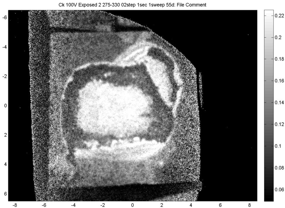
Figure 9-9 – Pseudocolored hyperspectral image of MC-exposed, fully-formulated MIL-PRF-85285, bottom surface, with brightness linked to C=C \pi^* peak area.
