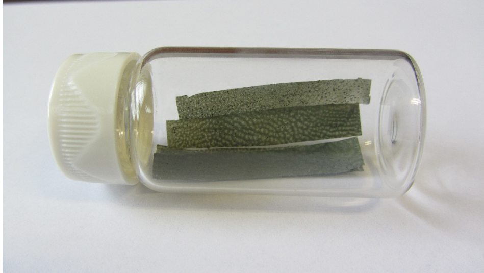
Figure 12 Strips with dimension 3mm width and 40mm length
