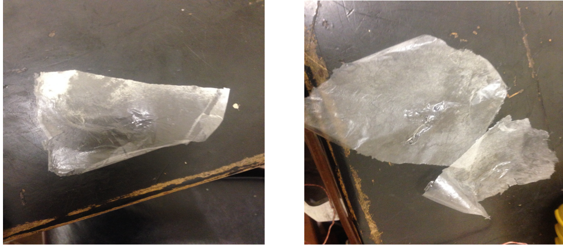
Figure 9 The sample of poorly dried fibers
