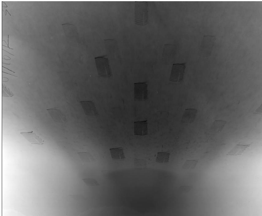
Figure 28: Scan of X-ray topography film with x-axis rotating 2.3 degree
