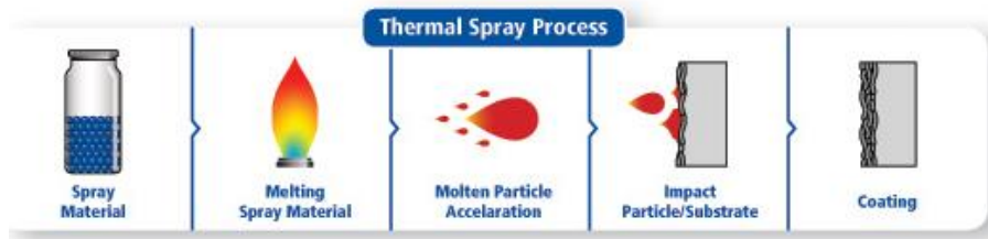
Figure 3.1 Principle of thermal spraying [109]
