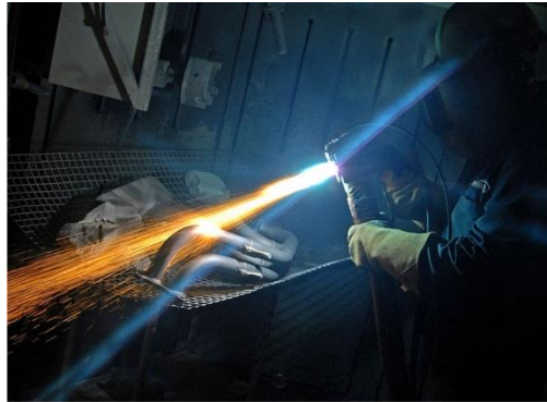
Figure 3.8 Plasma spray setup (Courtesy of Zircotec)
