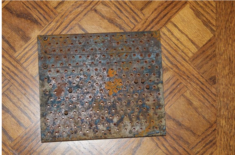
Figure 4.3: The jig plate used to hold nitinol wires during heat treatment. One of the benefits of this set-up is that the nitinol wire is held tight enough to go through several heat-quench cycles without loosening the wire. Wires can also be stacked on top of each other by using longer screws and spacing between them with nuts. Point A shows a nitinol wire prepared for heat treatment.
