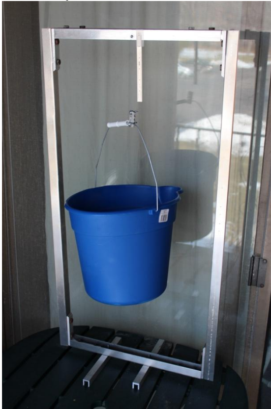
Figure 4.4: Experimental set-up for stretching wires. Machinist rule and nitinol wire are visible at the top.
