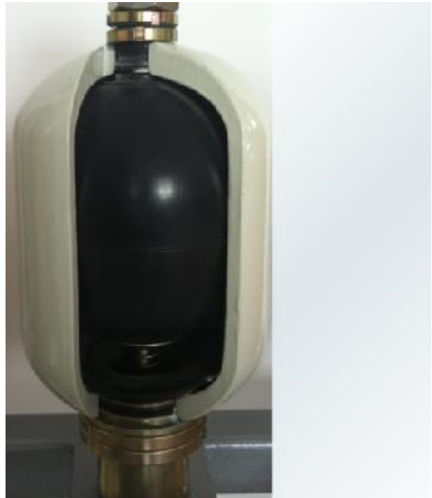
Figure 5.1: A cutaway view of a hydraulic-bladder accumulator. The parts of the hydraulic accumulator are: A) the steel casing, B) the nitrogen filled bladder and C) the oil storage area.
