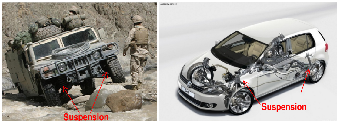
Figure 1. 2 Different suspension systems with emphases on steering and comfort (The pictures are from: United States Department of Defense gallery and http://blogs.km77.com/arturoandres/514/prueba-de-consumo-7-volkswagen-golf-vi-1-4-tsi-122-cv-dsg/ )
