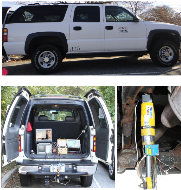
Figure 3. 14 Setup of the vehicle, instruments and sensors for road tests
