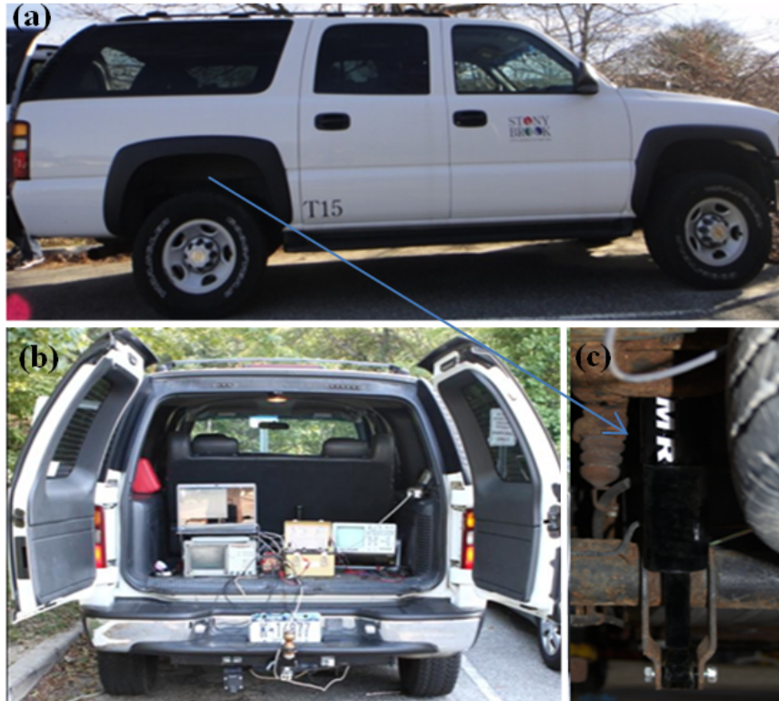
Figure 4. 18 The road test setup for the MMR shock absorber, (a) test vehicle Chevrolet Suburban SUV, (b) measurement equipment in the vehicle. (c) MMR shock absorber mounted on the left rear suspension.
