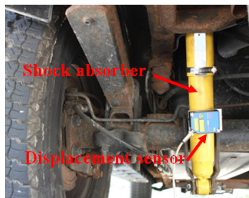
Figure 1. 6 Experiment setup for suspension vibration tests
