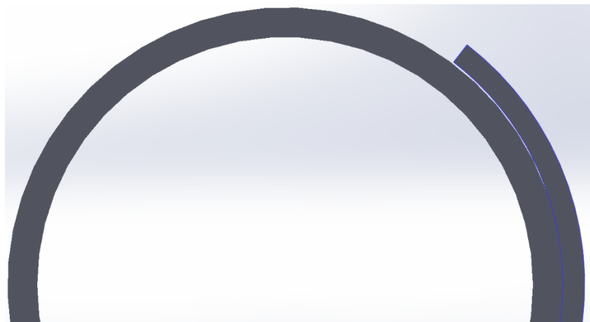
Figure 6-13 Gap between coupler and steam pipe after thermal expansion
