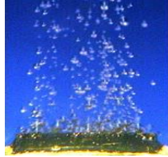
Figure. 8.3.2: Enforcing pool boiling heat transfer by reducing film formation on rough surfaces ( http://isnps.unm.edu/research/facilities/ )
