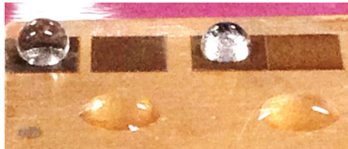
Figure. 2.2.2: Photograph of water droplets contact with copper surface. (Higher contact angle were achieved on laser-structured copper surfaces than on original untreated surface).
