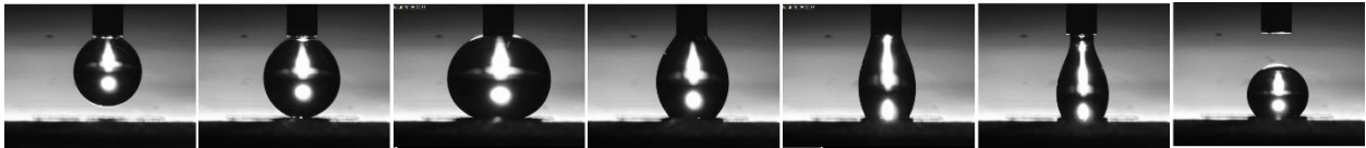
Figure. 5.7.2: Microscope images of water attracted to stay on the surface of high hysteresis. (2.3W of data set No. 1 on stainless steel)
