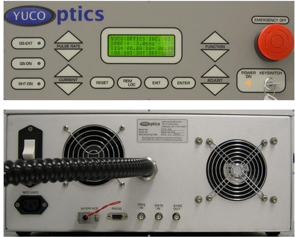
Figure. 4.1.2: Photograph of the laser controller front (upper) and back interface (lower).
