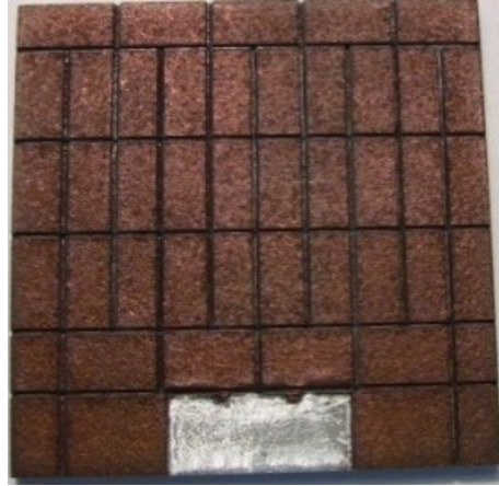
Fig. 5-4 Patterned bottom copper electrode on a flat substrate
