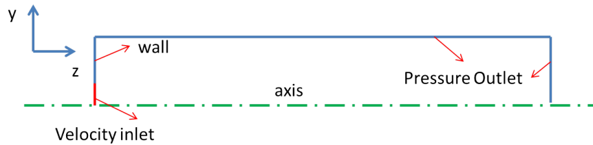
Figure 5.52: The boundary conditions for the two dimensional mercury jet simulation
