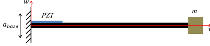
Figure 5.1 Flexible-beam structure with PZT film
