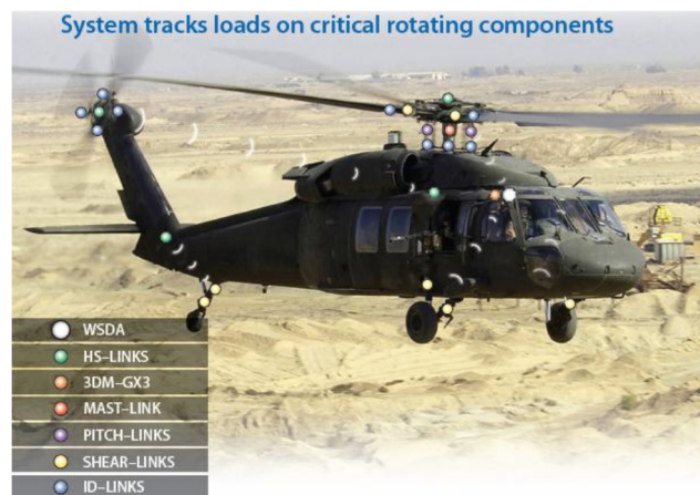
Figure 1.7 MicroStrain’s SHM sensors in helicopter application [27]
