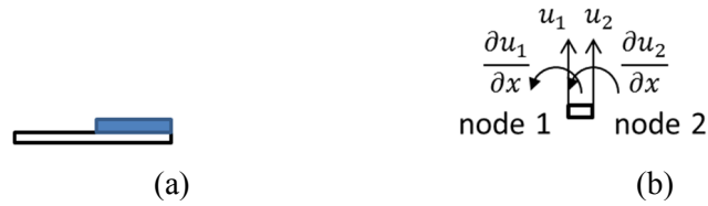
Figure 6.2 Beam metamaterial, (a) unit cell, and (b) each element with two nodes, each node has two coordinates
