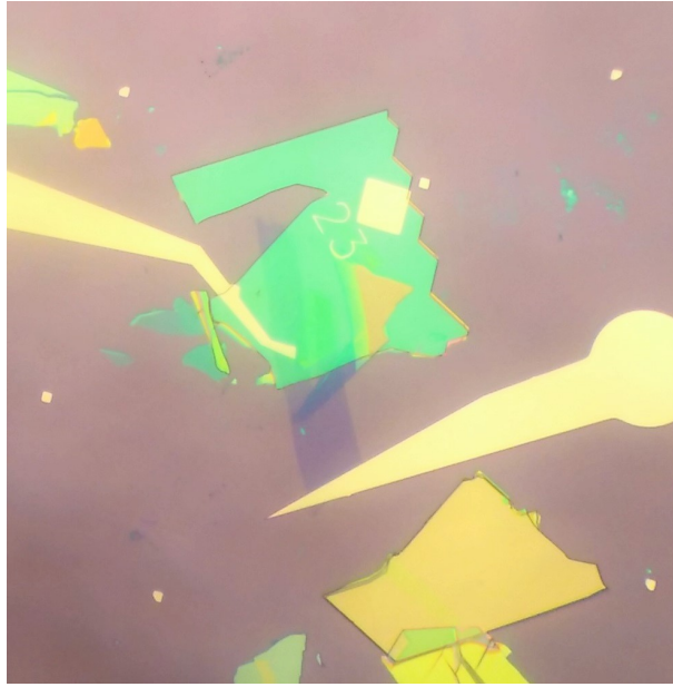
Figure 13: Optical image of a hBN graphene heterostructure as the schematic set up in Fig. 11. The graphene sandwiched by hBN is transparent but the location is extended out to the yellow colored electrode extended on top of the hBN (light blue) and the top hBN (slightly yellowish). Note that the top hBN is also very transparent due to its thinness ( \sim 5\text{nm} ) the bottom graphite (purple) is the bottom gate crossing partially the sandwiched graphene. Note that there is a fork like underneath the graphene sandwich.
