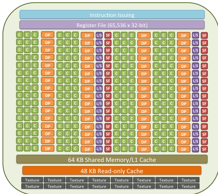
Figure 5.2 Schematic of an individual K20X SMX. See text for details. Image credit: Oak Ridge National Lab, Accelerated Computing Guide
