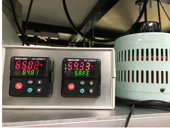
FIGURE 4.2: Temperature control box: the left sensor is connected to the heater while the right detects the cell's temperature. The two controllers are part of a feed-back electronics system to maintain the cell temperature around 60^{\circ}\text{C} at equilibrium.
