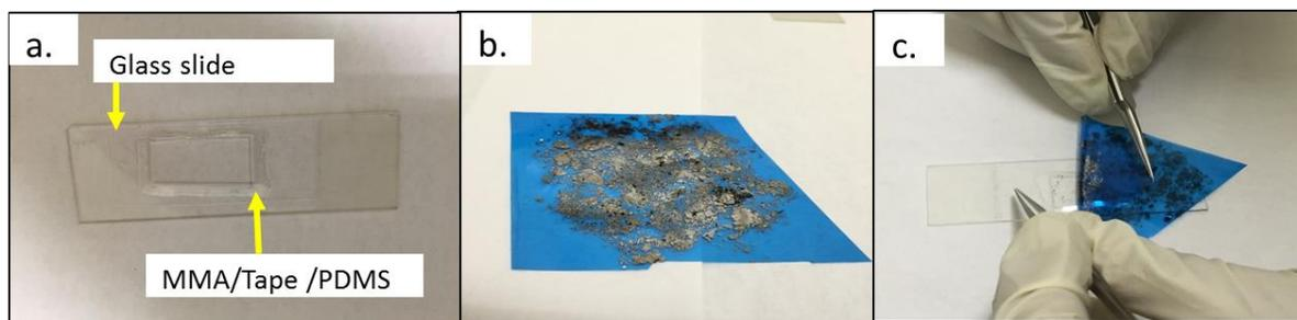
**Figure 5.6: Source substrate preparation.** **a.** Glass slide with MMA/tape/PDMS **b.** Graphene on blue tape ready for deposition **c.** peeling off tape after tape is pressed on the MMA/tape/PDMS substrate.
