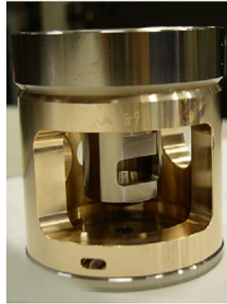
Figure 2.2 - Photographs of the objective pole pieces of a JEOL 3000F and JEOL 2100F Lorentz TEM. The 3000F consists of a symmetric pole piece design with a small gap, while the 2100F Lorentz TEM is composed of a mu-metal cage with a side entry port, creating a near field free specimen region.
