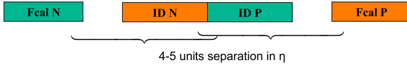
Figure 3.2: Illustration of the sub-FCal method. The tracks at positive \eta are correlated with FCal N and those at negative \eta with FCal P .
