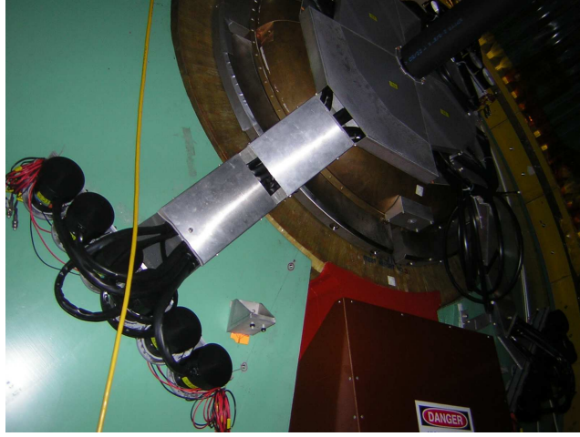
Figure 2.7: A picture of one of the quadrants of the RXNP detector installed on the face of the central arm magnet. The black pipe near the top of the picture is the beam pipe.
