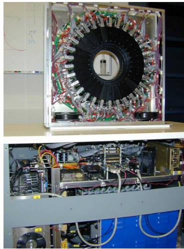
Figure 21: The microPET II scanner 61 (©2002 IEEE)
