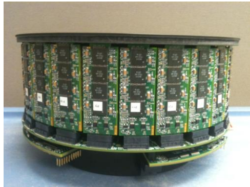
Figure 4: The Whole-Body Rodent PET Scanner (BNL-UPenn System) 7 (©2012 IEEE)
