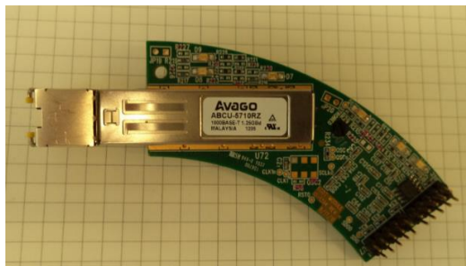
Figure 24: The updated Time Stamp and Signal Processing Module (TSPM), with SFP module attached)
