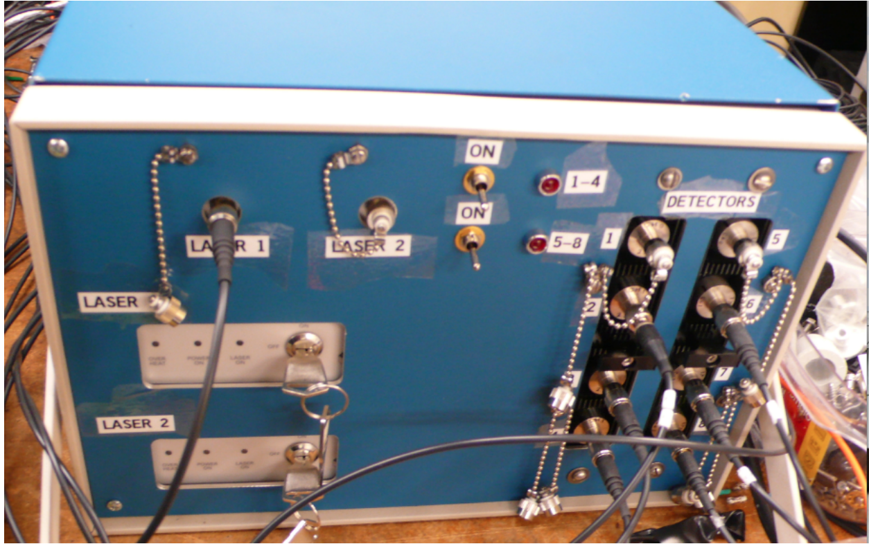
Figure 3.4: The front panel of the DCS module built in our lab at Stony Brook, showing two laser input sources (top left) and their power supplies (bottom left), and eight avalanche photodiode detectors (right) that are turned on and off using two toggle switches (center).
