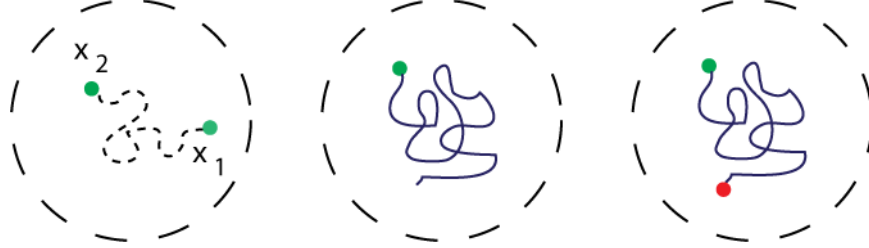
Figure 39 - Schematic of Fluorescence Correlation experiments on end-labeled polymers. (left) Pure diffusion; (middle) Single end-label; (right) Double two-color end-labels.
