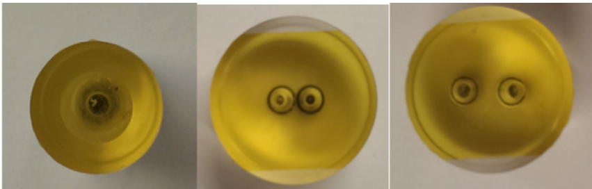
Fig.52 Three phantoms used for detector studies: Left: 10 mm cylindrical hole, Middle: 2 mm holes separated by 6 mm Right: 3 mm holes separated by 10 mm. Yellow surface is 25 micron thick kapton window.
