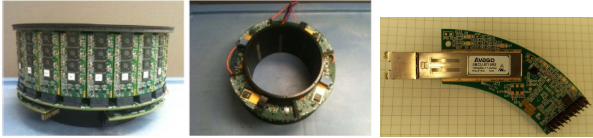
Fig.14 (Left) Side view of the scanner, without the side cover. (Middle) Bottom view of the scanner, displaying four TSPM boards without SFP modules, plastic clamps are design to hold the SFP modules from pulling by the magnetic field, (Right) TSPM board with SFP module plugged in.
