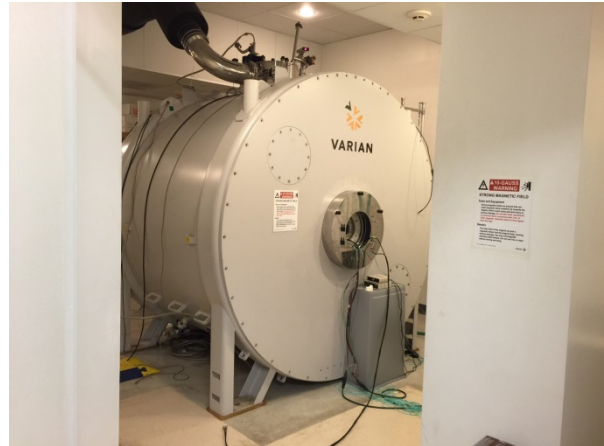
Figure.8 (left) Schematic of construction of a cylindrical superconducting MR scanner (image obtained from Wikipedia, free to reuse); (right) Varian 9.4T MRI in University of Pennsylvania
