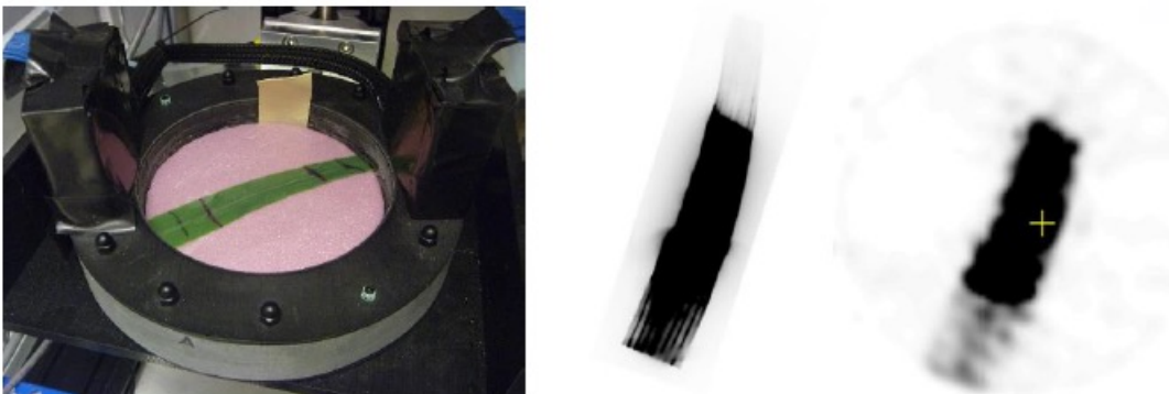
Figure.48 (left) A corn leaf which was cut one hour after ^{11}\text{C} -carbon dioxide uptake. (Center) A radiographic image of this leaf. (Right) a PET image taken with the BNL-plant scanner[88](©2013 IEEE)
