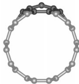
Figure 3: Stone-Wales defect in carbon nanotubes. Adapted from Reference 61 with permission. Copyright © John Wiley and Sons, 2005
