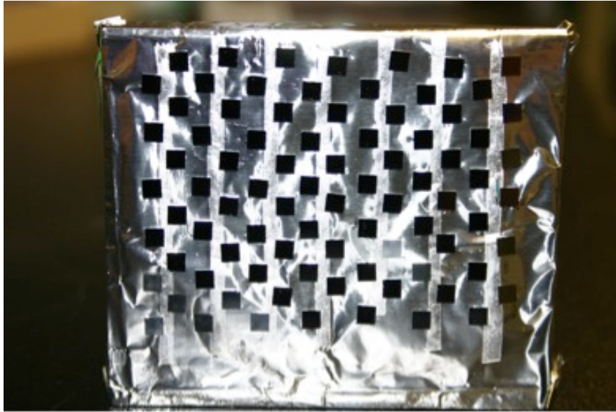
Figure 5.1. Silicon wafers attached to aluminum foil to be wrapped over the target plate of the electrospinning apparatus.
