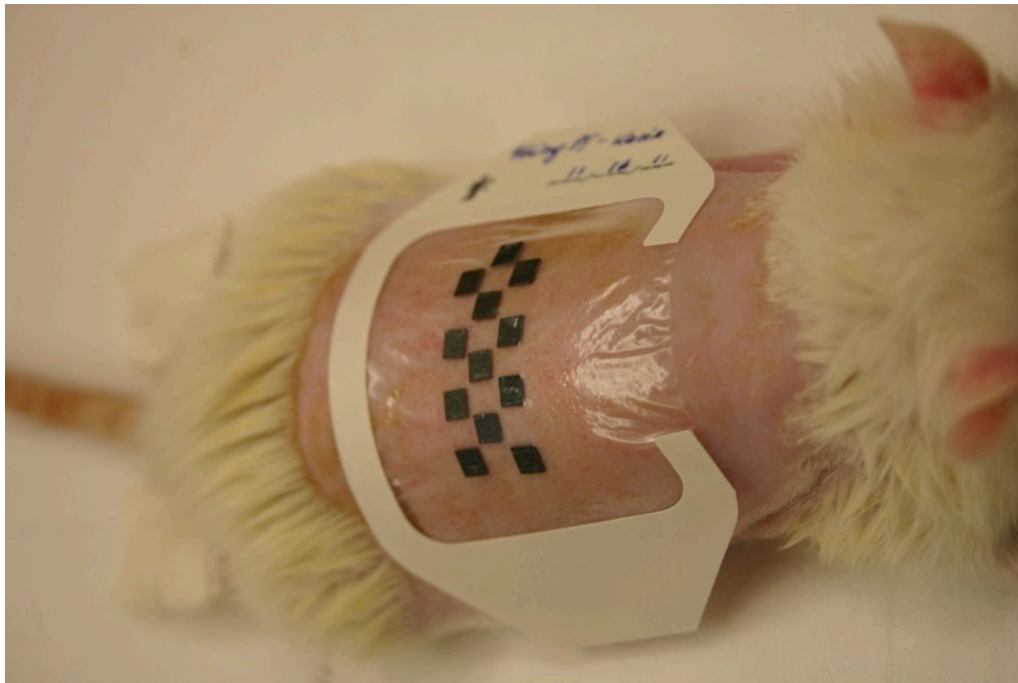
Figure 5.4. The PT-patch after application to the depilated dorsal surface of a rat; the sturdy backing material on the Tegaderm film was removed once the film was applied to each animal's back.
