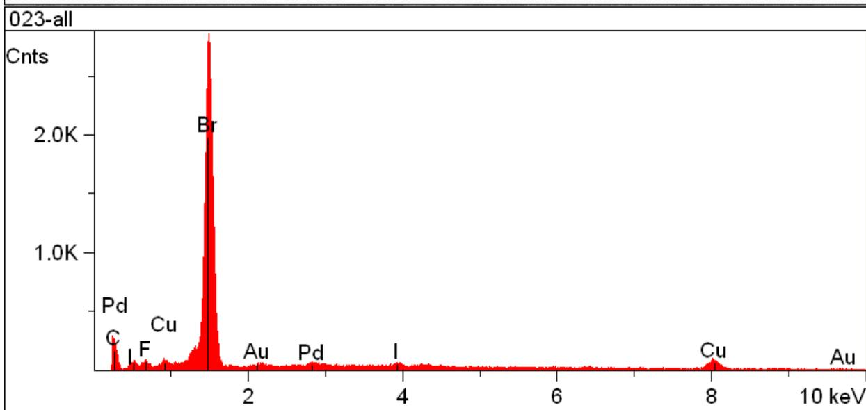
**Figure 4.4** SEM and EDS spectrum of reacted PBDA cocystal after Suzuki Reaction
