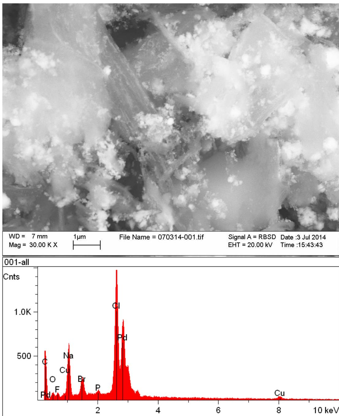
**Figure 4.2** SEM and EDS spectrum analysis of black power after purification
