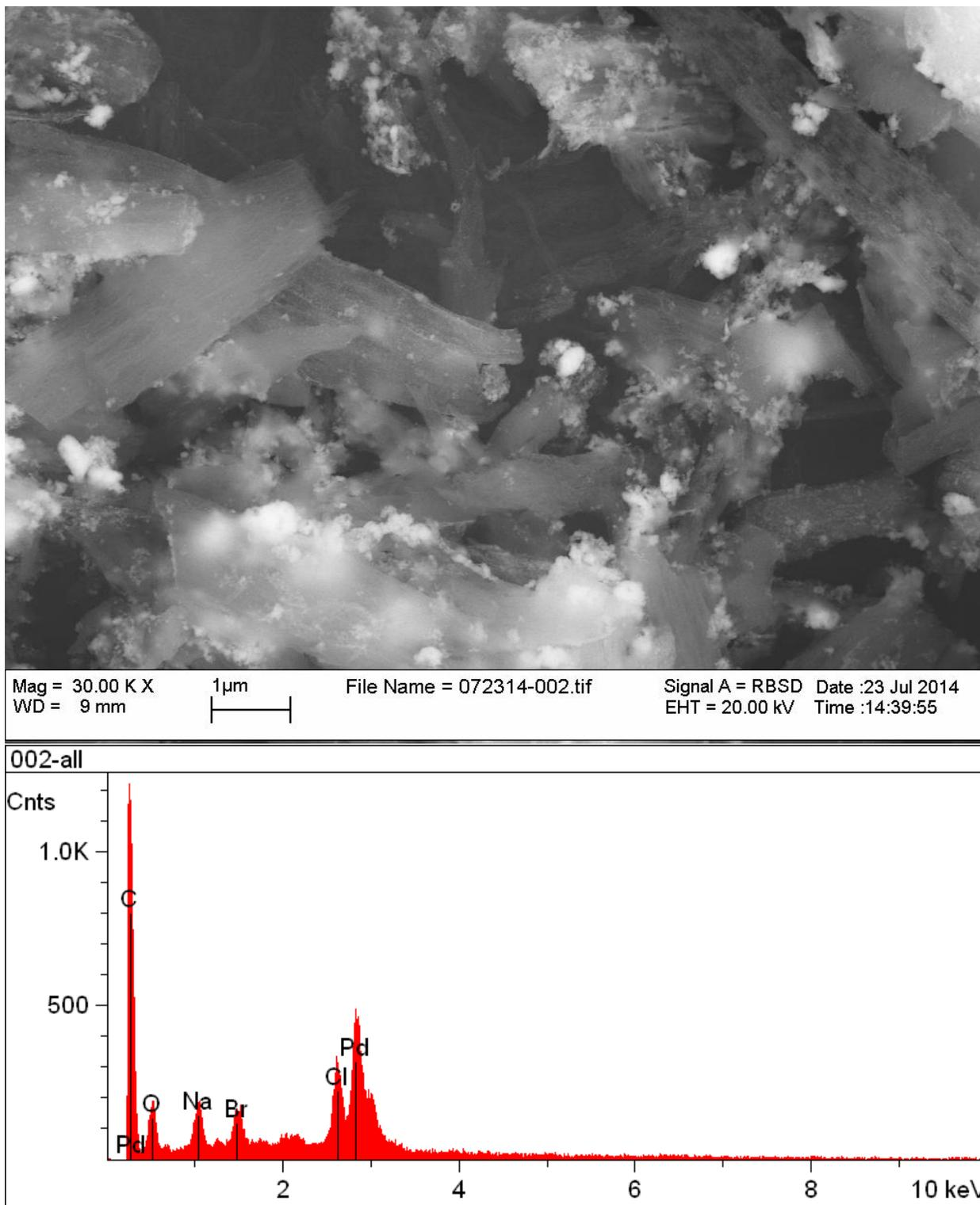
**Figure 4.3** SEM and EDS spectrum analysis of black power after purification
