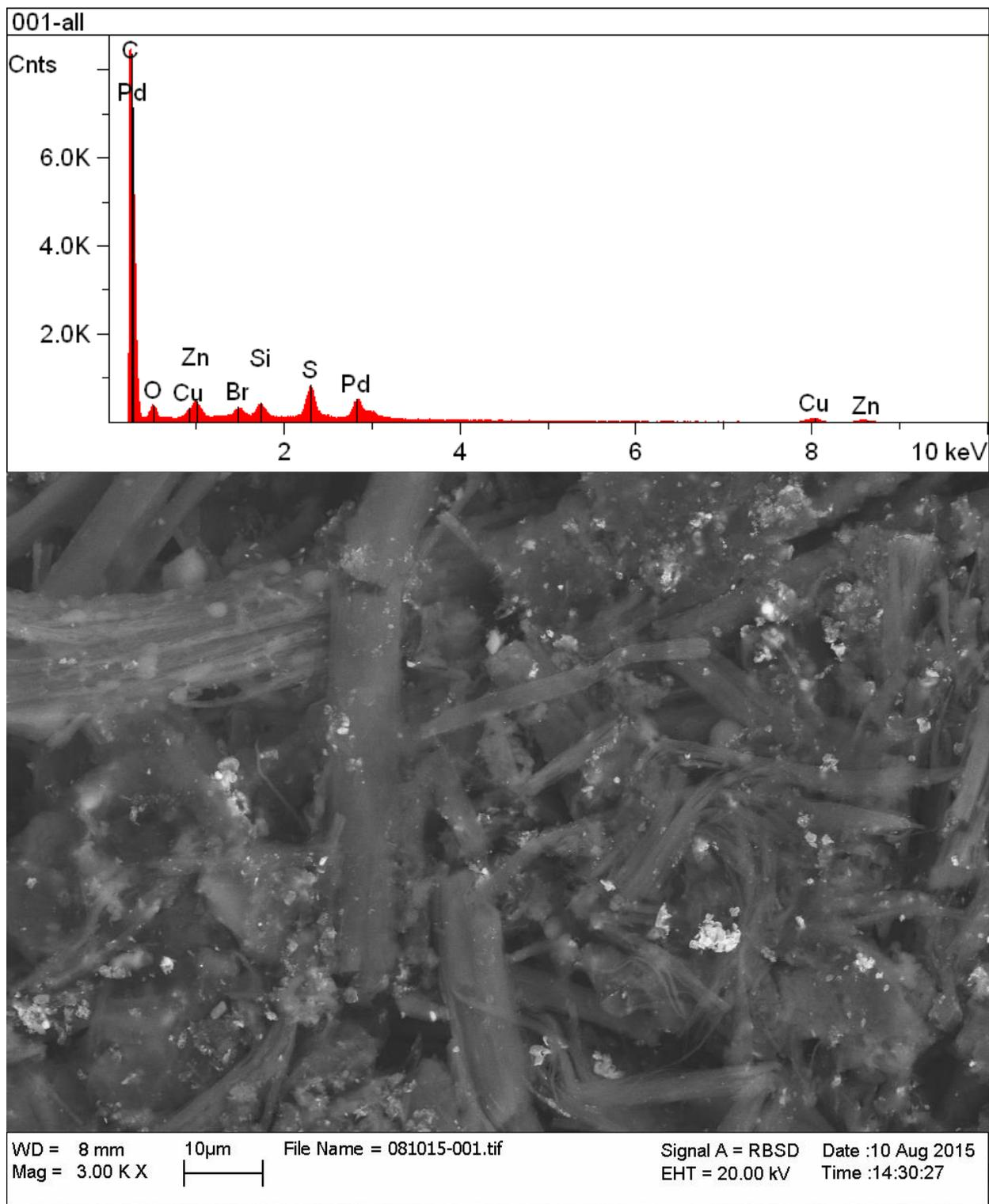
**Figure 4.6** SEM and EDS spectrum of reacted PBDA cocystal after Sonogashira Reaction
