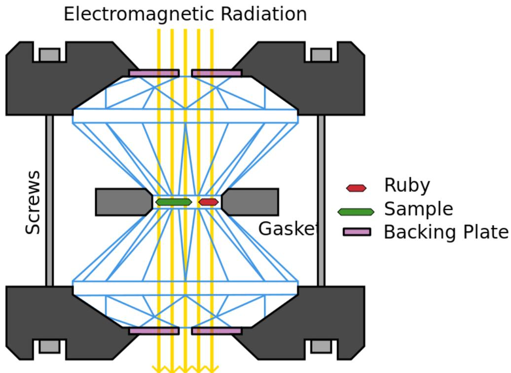
**Figure 2.1** The structure of diamond anvil cell<sup>27</sup>
