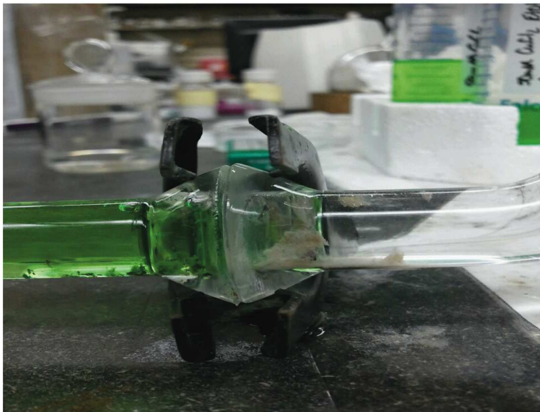
Figure 3.14. Image of as-prepared Cu NWs formed using a U-tube double diffusion device under ambient conditions. Nanowires were prepared using \text{CuCl}_2 in EtOH and a reducing agent, i.e. hydrazine, dispersed in EtOH. Supplemental information image reprinted with permission from Ref. 53. Copyright 2014 American Chemical Society.
