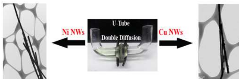
Figure 1.7. Schematic of the U-tube double diffusion technique for the synthesis of Cu and Ni NWs. Image reprinted with permission from Reference 66. Copyright 2014 American Chemical Society.
