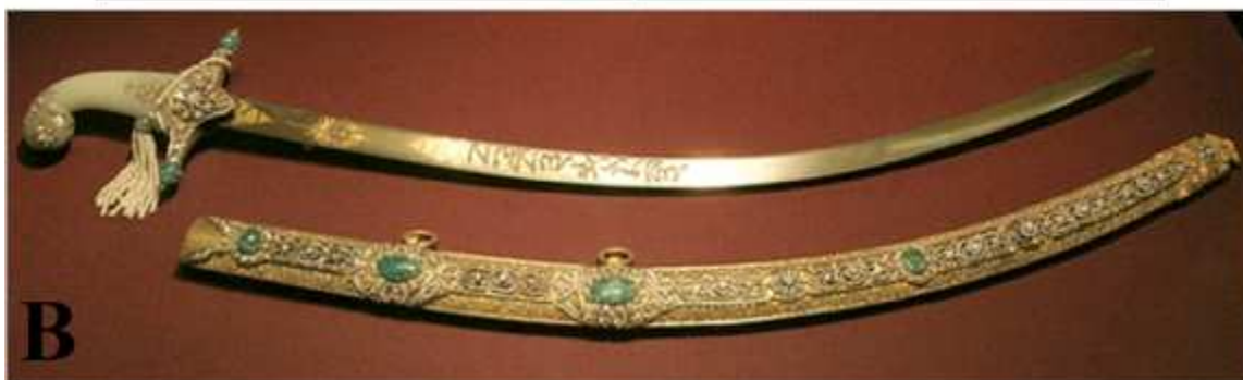
Figure 1.3: The Lycurgus cup at the British museum lit from the outside (A) and the inside. A Damascus Saber (B) composed of carbon nanotubes and cementite nanowires (photo by Tina Fineberg for the New York Times).
