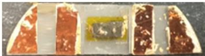
Figure 1.14. The set up for a four-probe electrical resistivity measurements is shown. The bar shaped sample (gray) is mounted on a sapphire stage with double sided Kapton tape. The Cu pads (orange) are connected to the sample via thin Pt (black) wires and silver epoxy. Each Cu pad is connected to an external source meter using metal-to-metal pressure contacts. The actual experimental setup is also displayed.
