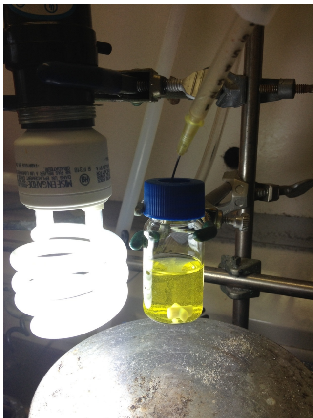
Figure 4.8. Visible light photocatalysis reaction set-up.
