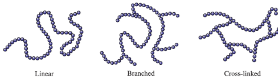
Figure 1.15 Linear, branched, and cross-linked arrangements in a polymer 19 .
