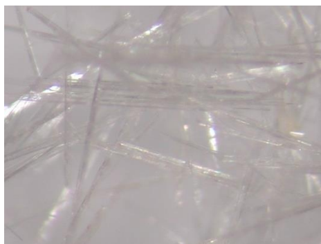
Figure 2-35. Needle like crystals of M11 obtained after crystallization
