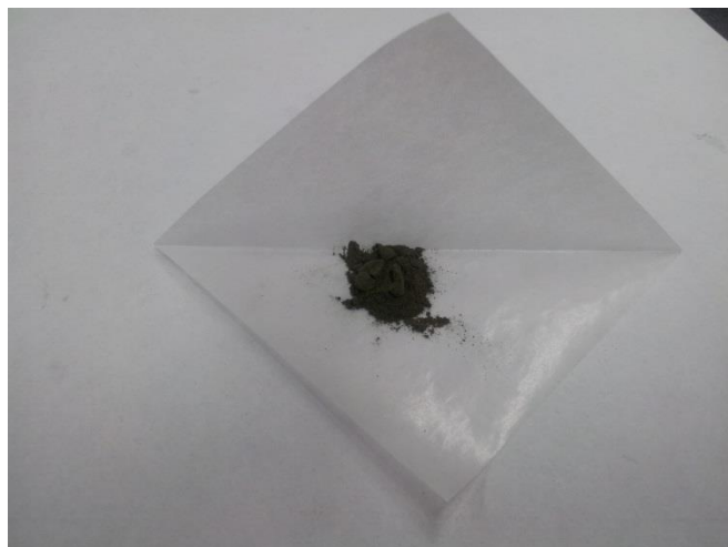
Figure 10. The olive-green ordered Na(Ni 2/3 Sb 1/3 )O 2 powder.
