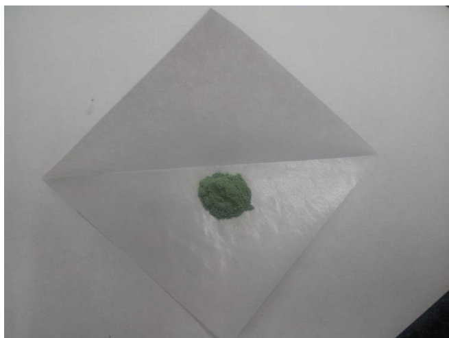
Figure 8. A light green powder sample of disordered \text{Na}(\text{Ni}_{2/3}\text{Sb}_{1/3})\text{O}_2 .
