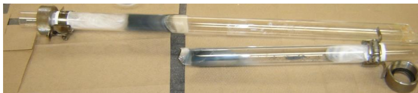
Figure 2.1. Effects of zinc volatilization on reaction apparatus components.
