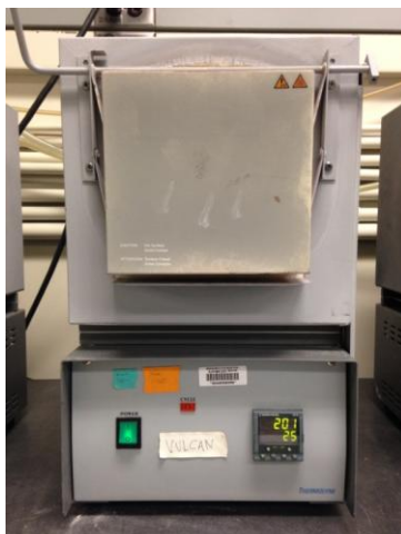
Figure 14: Thermo Scientific™ Thermolyne™ air furnace used in the synthesis of \text{InPO}_4 .
