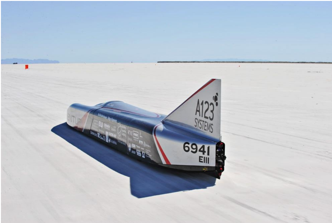
Figure 1: The Buckeye Bullet Electric Streamliner used A123 Systems' \text{LiFePO}_4 batteries to set a land speed world record of 307.66 mph. Photo credit: http://www.a123systems.com/lithium-iron-phosphate-battery.htm .
