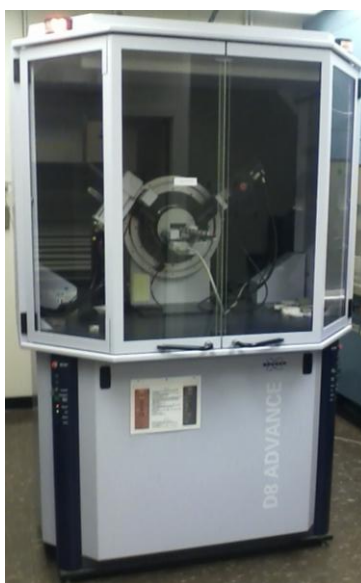
Figure 15: Bruker-AXS “D8 Advance” powder diffractometer used for PXRD pattern collection.
