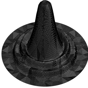
Figure 5.20: Cross section of numerical solution of \rho in xy plane of 3-D explosion test with third-order WLS-ENO at t = 0.1 .
