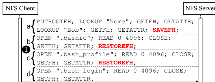
Figure 3.3: One NFS compound that reads three files. The operations can be divided into four groups: (a) sets the current and saved filehandle to /home/Bob ; (b), (c), and (d) read the files .bashrc , .bash_profile , and .bash_login , respectively. SAVEFH and RESTOREFH (in red) ensure that the CFH is /home/Bob when opening files. The reply is omitted.
