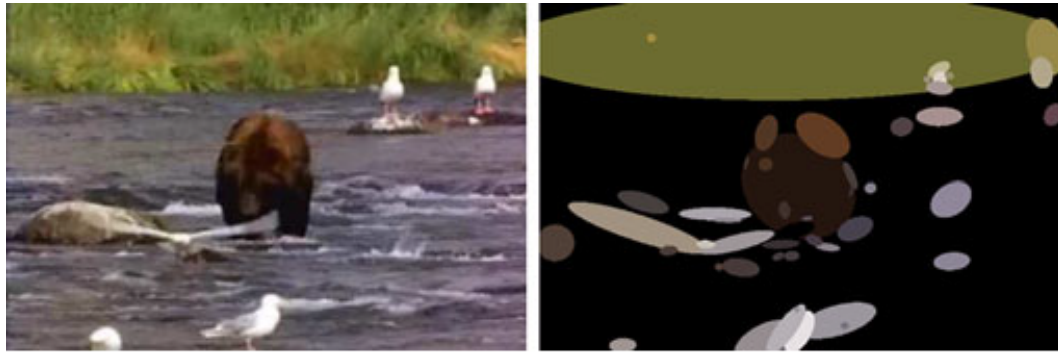
Figure 2.4. Left: input image; Right: proto-object in color blob representation using color blob detector from [49]. Image source [168].
