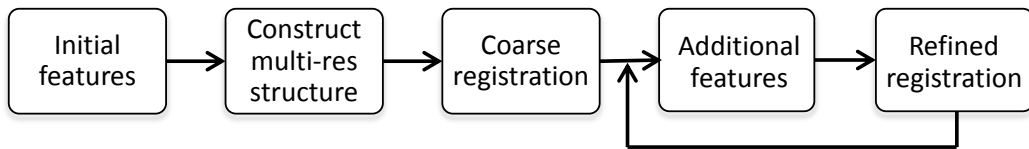
Figure 6.6: Pipeline overview of our hierarchical registration framework.
