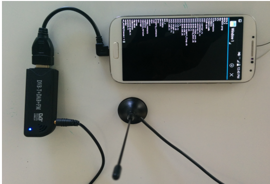
(E) RTL-SDR with Samsung Galaxy S4
