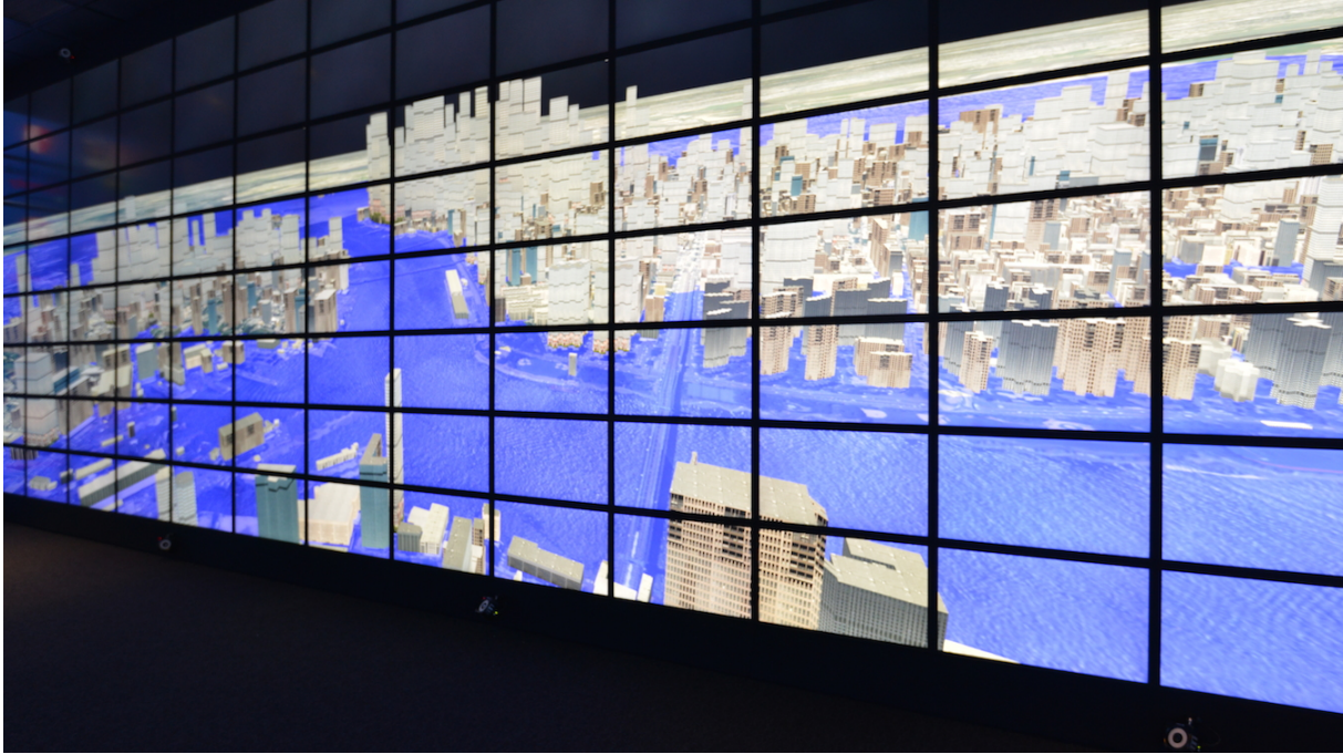
Figure 20: Immersive 3D ADCIRC simulation visualization. Illustration of simulated flooding in down-town Manhattan, generated via our extensions to osgEarth which permit interfacing with ADCIRC simulations.
