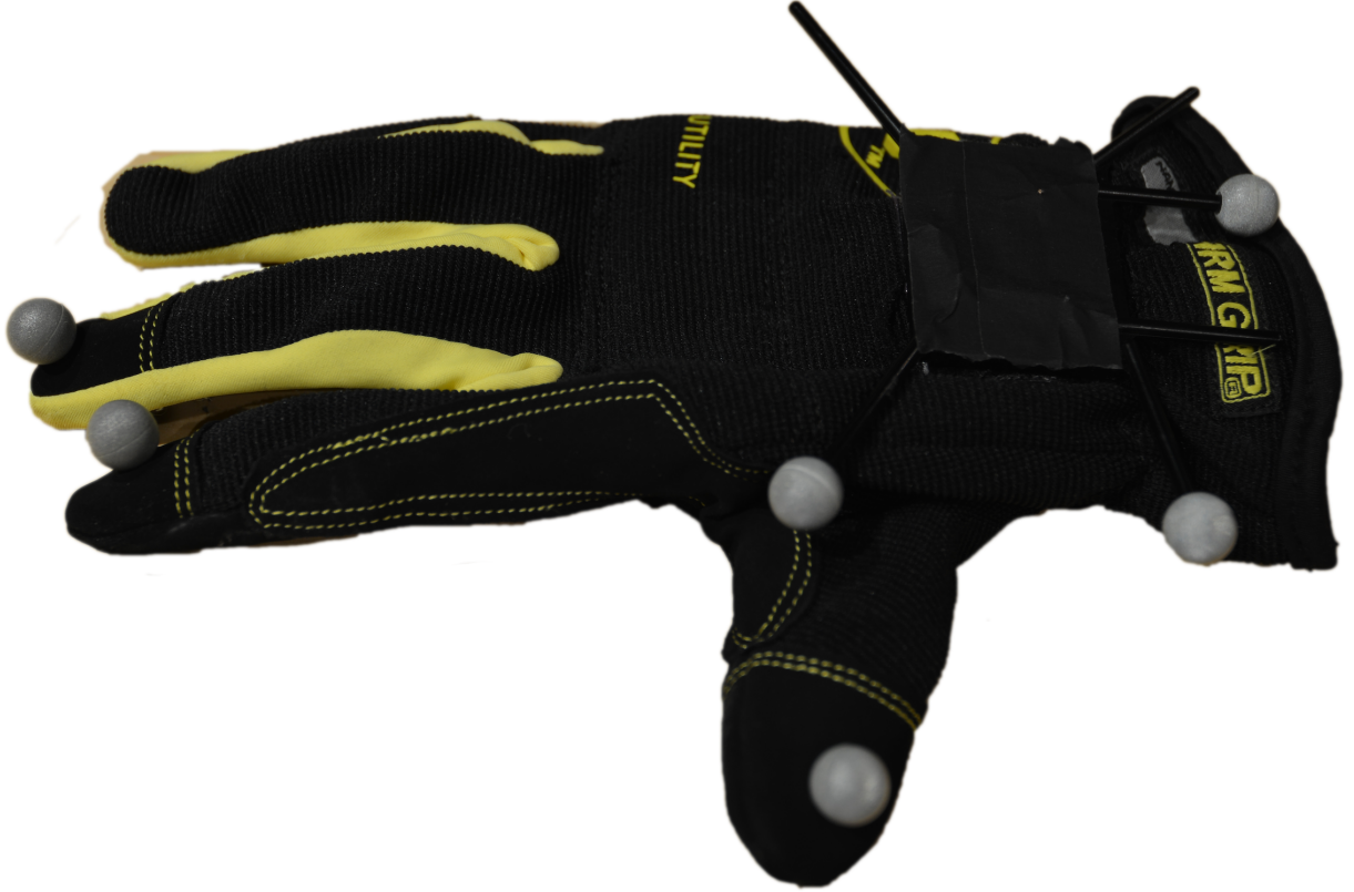
Figure 29: Low-cost, passively tracked gloves used by chirocentric user interface. It is constructed by attaching a tracking system rigid body to the back of a soft glove, using wires running through the fabric to preserve its elasticity and ensure a deformation-resistant connection. Retroreflective markers are attached on the tips of the thumb, index and middle fingers. The total cost of materials for one glove is under $25.
