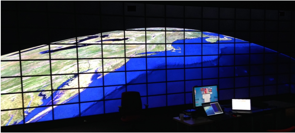
Figure 17: Zoomed-out view of the earth from our 3D GIS renderer. The base map layer was streamed from Mapquest Open.
