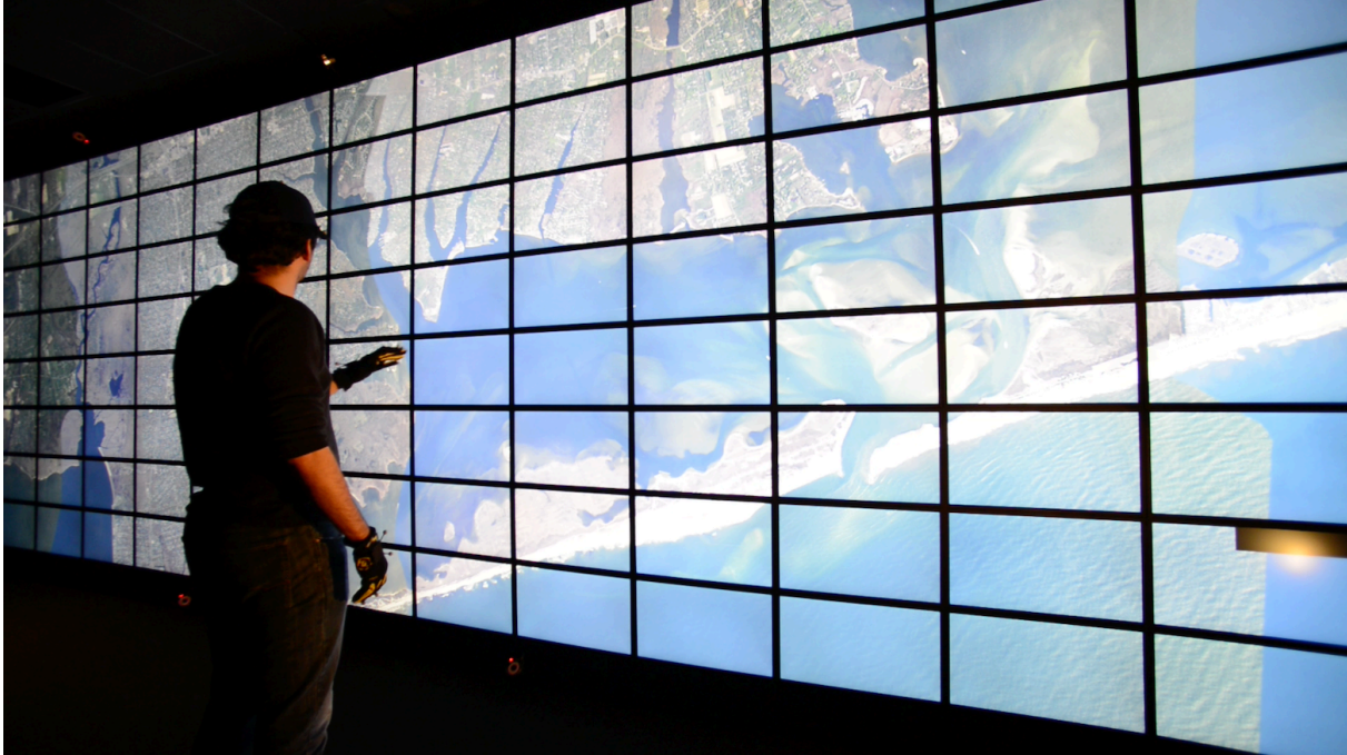
Figure 34: Photograph of a user leveraging our chirocentric user interface. The user is exploring a 2D GIS dataset in the Reality Deck. The rendering is generated with our VL-based renderer module.
