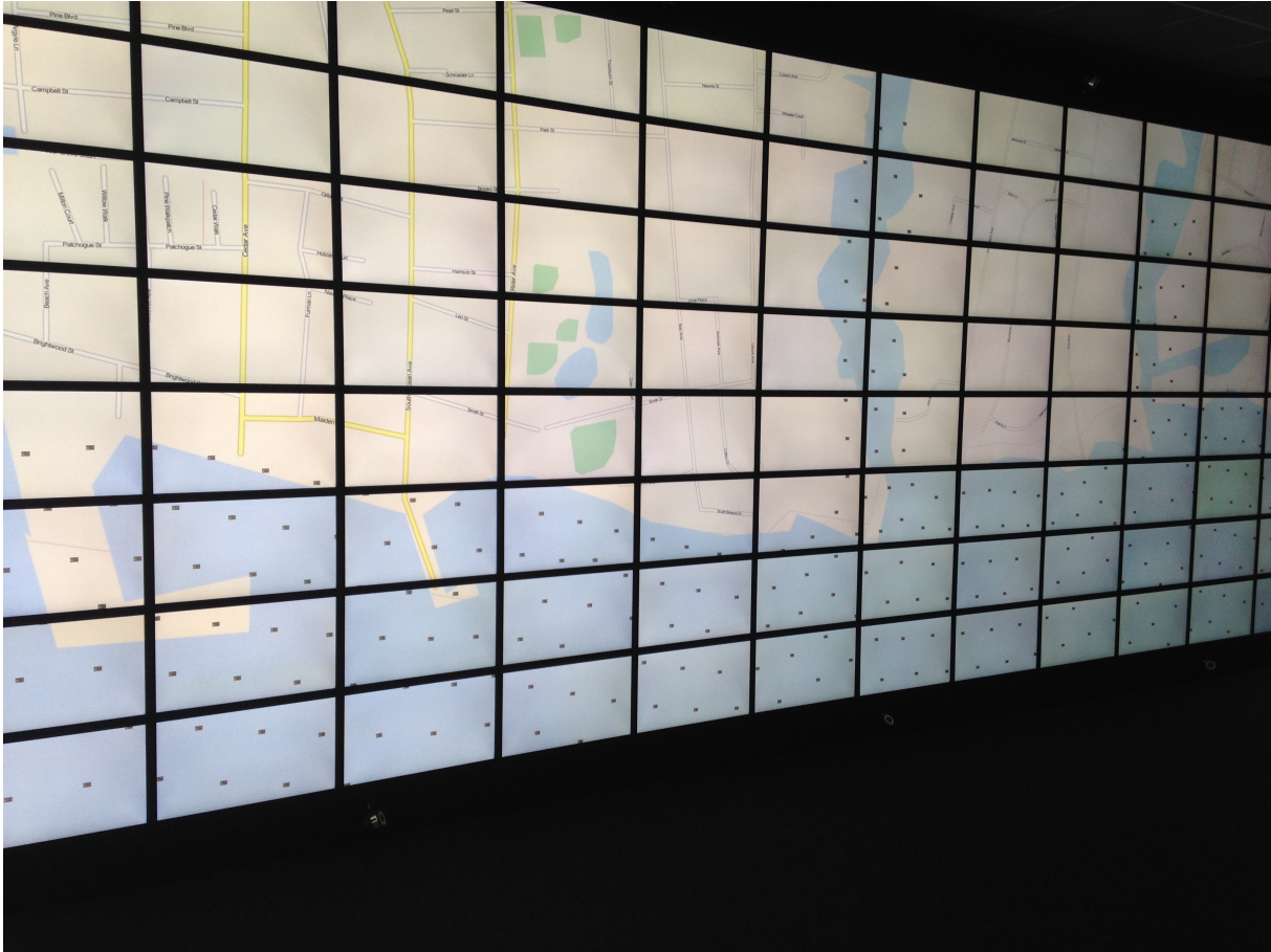
Figure 11: Example view of a 2D GIS scenario visualization. A scenario file was used to describe a visualization which includes a tiled based map streaming from Mapquest Open and a glyph data overlay driven from an ADCIRC simulation.
