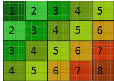
FIGURE 2.12: Execution pattern of the x86 based tiled-loop code. The numbers on the tile shows when a tile get executed. Tiles with the same numbers gets executed in parallel.
