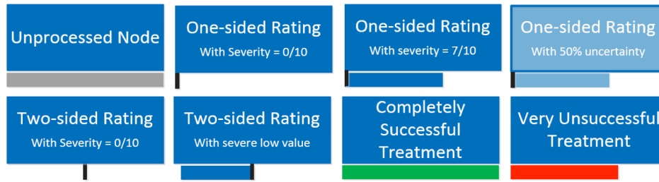
Fig. 5.8: Severity and uncertainty rating bar variations for sequential display nodes. The location of the vertical black line below the node indicates whether the data item is a two-sided rating (black line in the middle) or a one-sided rating (black line on the left). The length of the bar encodes the value and its saturation encodes the uncertainty of that value. The text inside the boxes above explains the semantics that our system uses in more detail.
