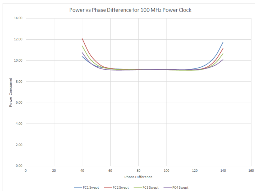
FIGURE 4.8: Overall power consumption in \mu\text{W} (summation of the power consumed by each power-clock signal) vs. phase difference (in ^\circ ) for 100 MHz power-clock frequency when only the phase difference of one power-clock signal varies (with respect to the following power-clock signal).
