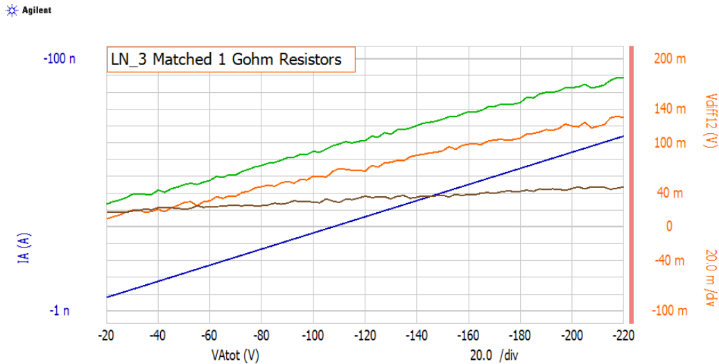
Figure 4.20: Series connection IV results for Ohmite 1G\Omega resistors at liquid nitrogen temperature
