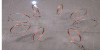
(b) Power a 14W lamp by organizing repeaters into domino form (courtesy of [78]).
