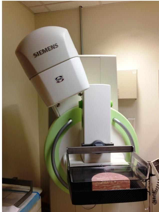
Figure 1.7 The Siemens Mammomat Inspiration DBT unit is shown with the phantom situated for acquisition. The compression paddle sits atop the phantom, and the phantom sits directly atop the carbon-fiber detector cover. The X-ray tube is housed in the top enclosure that rotates.
