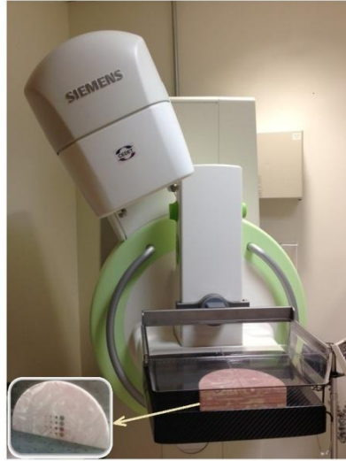
Figure 3.1 Siemens Mammomat Inspiration CEDET scanner used for acquisitions. A CIRS BR3D (model 020) phantom is shown mounted in the scanner. The inset shows a customized slab of the phantom with iodine inserts.
