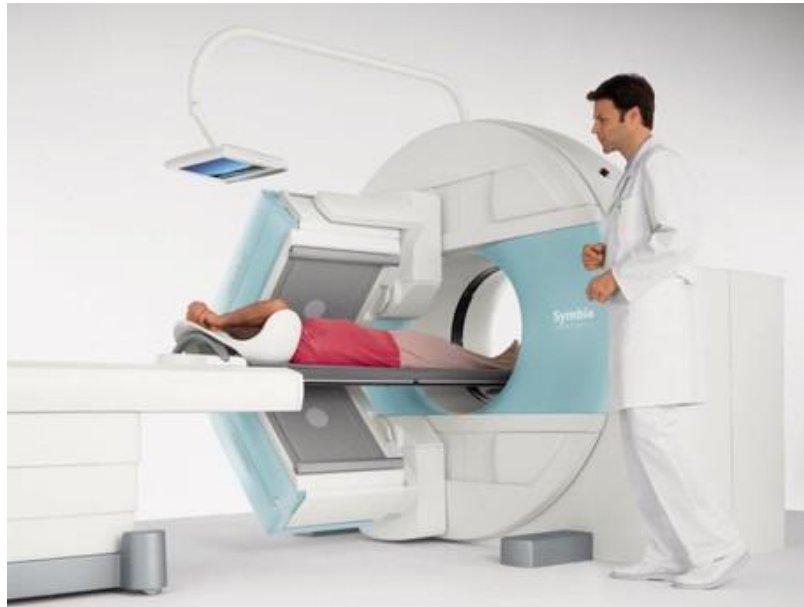
Figure 5.1 SPECT-CT scanner. The patient sits underneath the two SPECT camera units. The CT unit is the large circular structure. After the SPECT scan, the patient is imaged by the CT. Photo is in curtesy of Siemens Healthcare.
